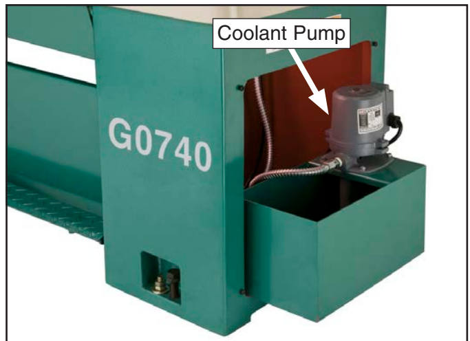
Figure 140. Coolant pump location.
